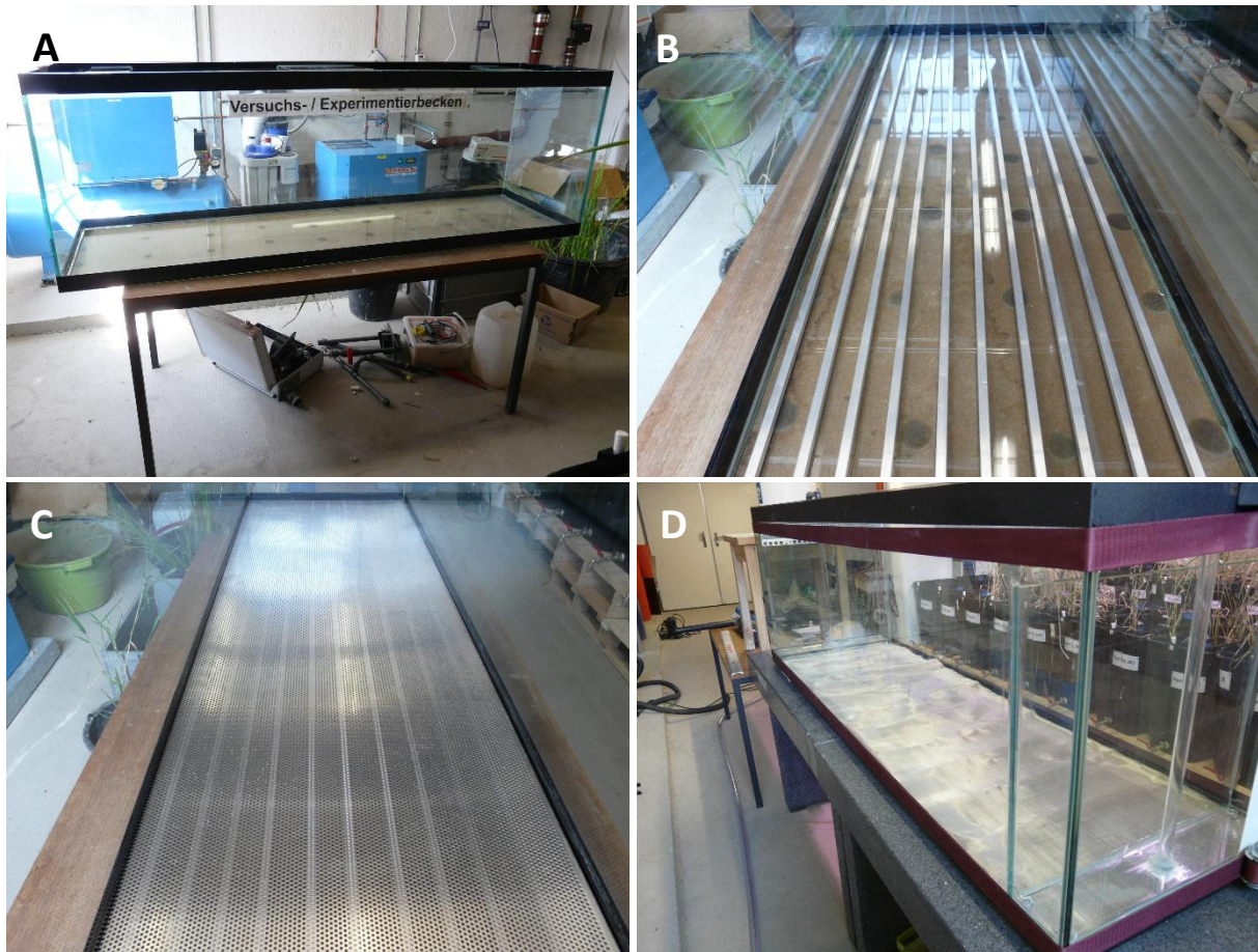
Figure 1. Different stages in the construction of the inlet and outlet reservoirs and sediment bed: A) front view of the aquarium before starting the construction of the model CW system, B) top view of the system with the square tubes made of aluminum, C) top view of the system with the aluminum perforated plate and D) perspective view of the system with the stainless steel wire mesh, the inlet and outlet reservoirs and the Plexiglas tubes.
