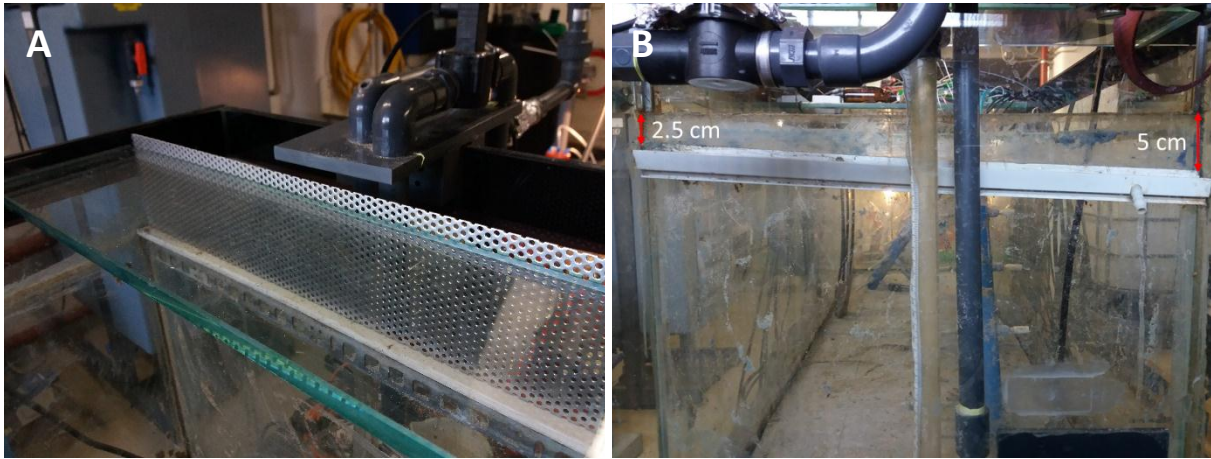
Figure 2. A) Aluminum perforated sheet placed on top of the glass wall at the inlet reservoir and B) water collector gutter-like with a small drain at one end for sampling purposes glued to the glass wall of the outlet reservoir.
