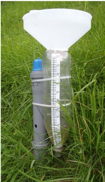
Figure 6: Rainfall collector with integrated measuring scale attached to the PVC well casing. This bottle was just emptied.
