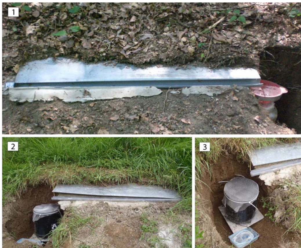
Figure 5: 1) Surface flow collector at the mixed forest hillslope. In the beginning, surface flow was collected in a canister. 2) Surface flow collector at the grassland hillslope after the installation of the tipping bucket. 3) Close-up of the tipping bucket, which is fixated on a steel plate leveled out by three poles.
