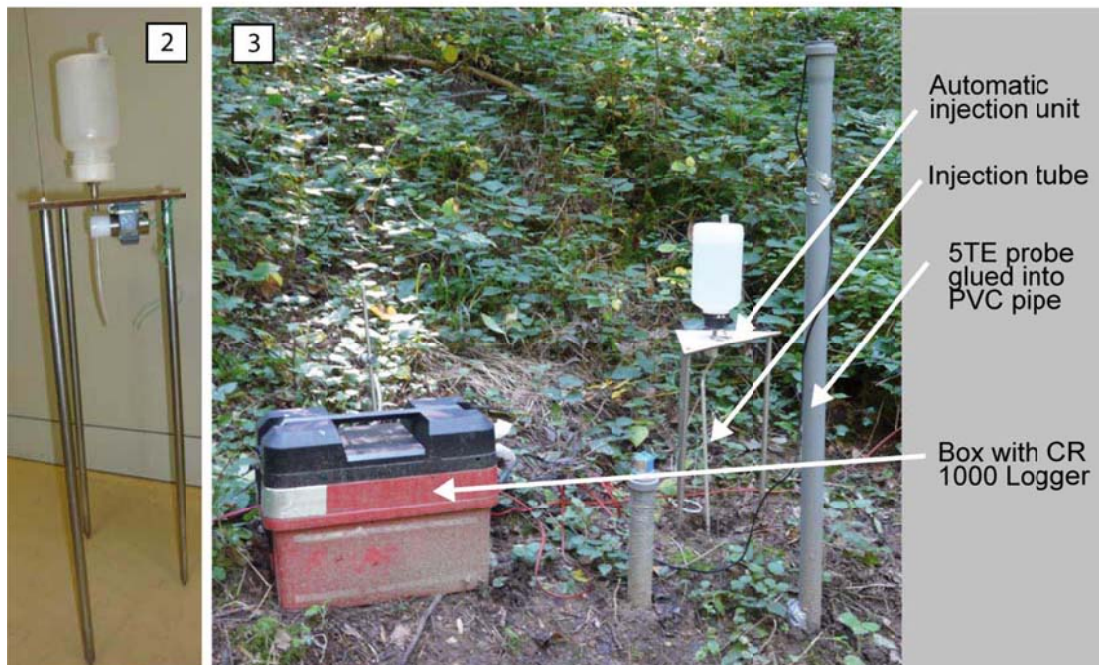
Figure 4: 1) Lab test in a sand filled box with constant in- and outflow conditions. 2) Design of automatic tracer injection unit (plug valve connected to a bottle with NaCl solution). 3) Set-up in the field.
