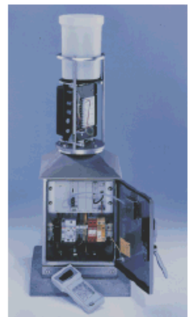
Fig. 3 Ombrometer Automatic raingauge
