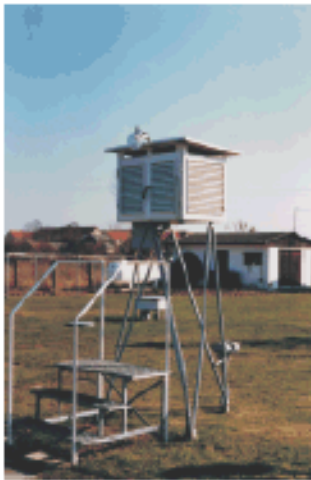
Fig. 2 Screen of a DWD climate station
