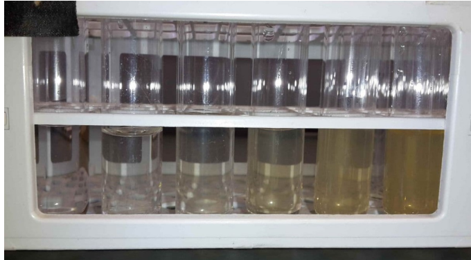
Figure 3.14: The serial dilution of sample 1 with 5, 10, 25, 50, 75 and 100% solution, that is used for the calibration.
