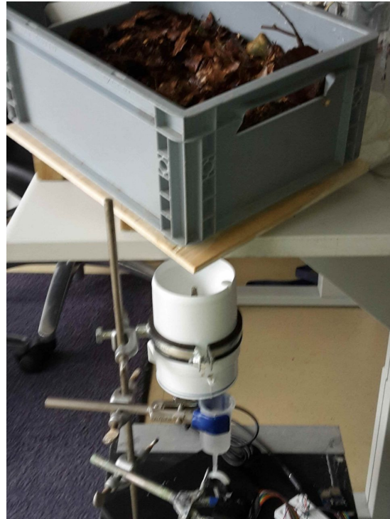
Figure 3.20: The box with the soil sample is placed on an inclined plane with holes in the low corner. Below the holes the measurement system of drop counter and spectrometer is positioned.
