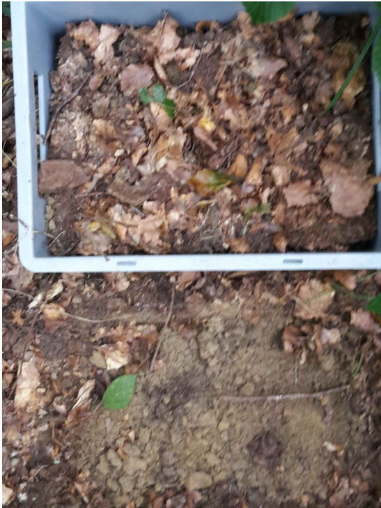
Figure 3.19: A block of soil the size of the plastic box is cut with a spade and put into the box.
