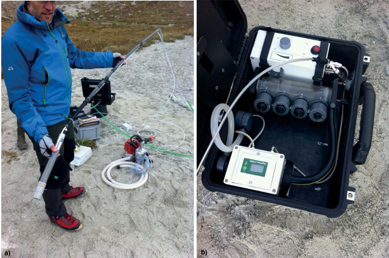
Figure 4.6: (a) Self-made double packer system with attached pressure sensor and electrical water pump. (b) Prototype of pumping devices.
