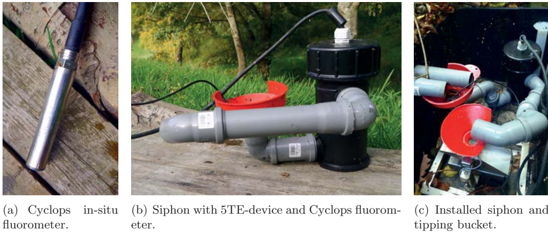
Figure 5: Measurement setup of the Cyclops in-situ fluorometer for uranine concentration measurement at the trenches N and W.
